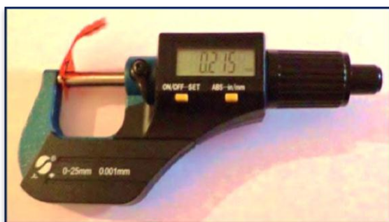
Figure 4: Measuring the thickness of the Duralay.
