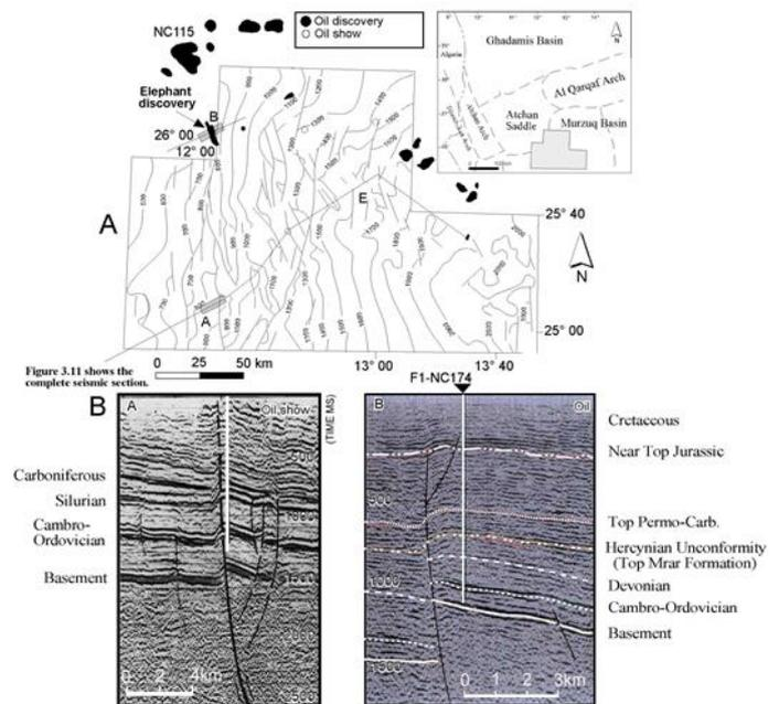
Fig. 7. A) TWT structural map (Middle Devonian unconformity), C.I.20 msec, showing N-S en-échélon fault blocks. The fault system is part of the 10° wrench zone. B) Seismic windows, the seismic sections showing flower structure in concession NC58 (window A) and reverse faulted anticline formed over a basement uplift (window B). Well F1-NC174 is a well in the giant Elephant field, while the other well is a dry hole in a smaller but well-defined closure to the south.
