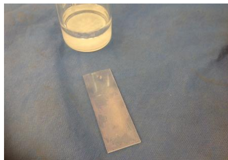
Fig. 2. Photograph shows of ZnS thin film formed at the water/toluene at 60^\circ C .
