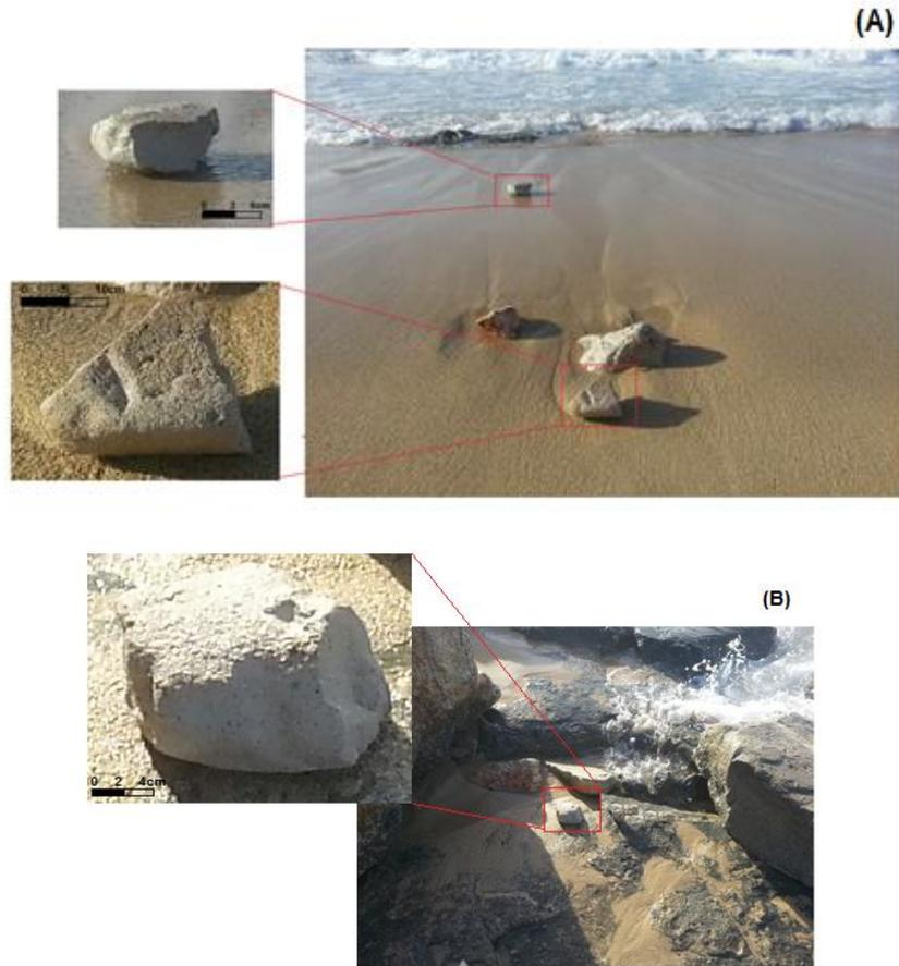
**Fig. 4.** Pumice rock fragments of various sizes and shapes with a vesicular texture (A: AT1- sample from the coast of At Tariyah, B: QL1-from the coast of Qasr Libya).
