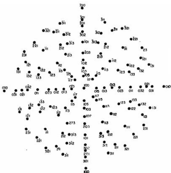
Fig. 3b. A map of location for the images of various planes when using a tube with a flat fluorescent screen.
