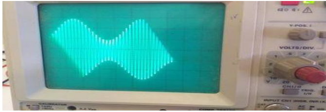
Fig. 34. The output amplitude modulated wave at point (b) after connecting the LC resonant circuit in Fig. 21 ( V_m = 6 V, V_c = 15 V).
