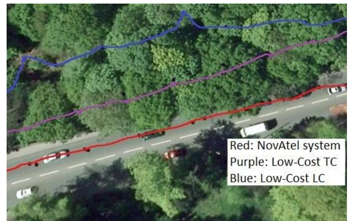
Fig. 13: GPS/INS integration with limited satellites.
