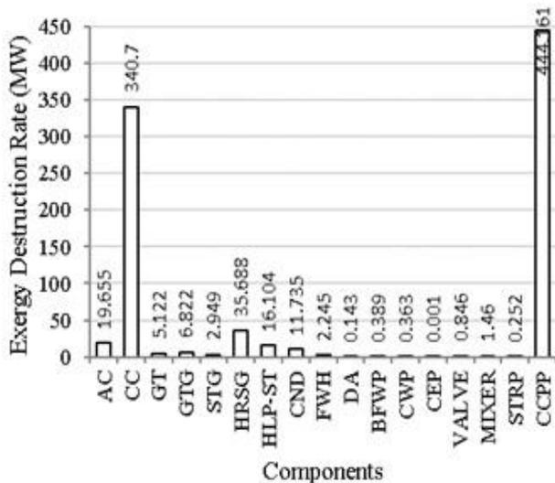
**Fig. 3:** Exergy destruction rate of the CCPP components.
