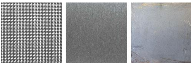
Fig. 3: Textured aluminium sheets (a) vertex: mill finish textured sheet, (b) flat plain aluminium sheet: anodised finish sheet and (c) sheet was made using the shot blast method
