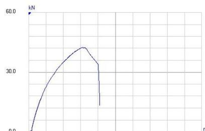
Fig. 9: Load-elongation Curve for S14.
