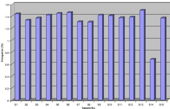
**Fig. 12:** Effect of Cathodic Protection on Elongation
