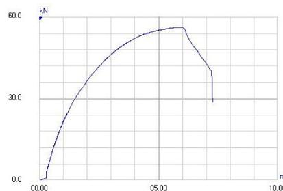
Fig. 10: Load-elongation Curve for S15.
