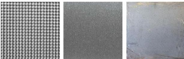
Fig. 3: Textured aluminium sheets (a) vertex: mill finish textured sheet, (b) flat plain aluminium sheet: anodised finish sheet and (c) sheet was made using the shot blast method
