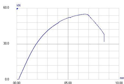
Fig. 7: Load-elongation Curve for S8.
