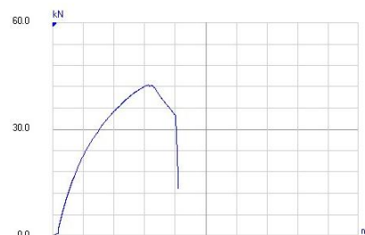
Fig. 9: Load-elongation Curve for S14.
