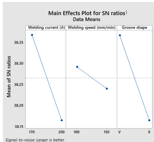
Fig.5. Main effect plot of S/N ratios for weldments hardness
