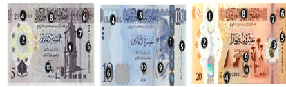
Figure (10): Basic features of data Libyan security banknotes. (1). Holographic Stripe. (2). Protection. Portrait, Clear Window. (3). SPARK on Secondary Window. (4). Magnetic numbering. (5). Fluorescent numbering. (6). Tactile Emboss. (7). engraved Gravure stripe. (8). Relief writing. (9). The prominent engraved landmark. (10). The signature
