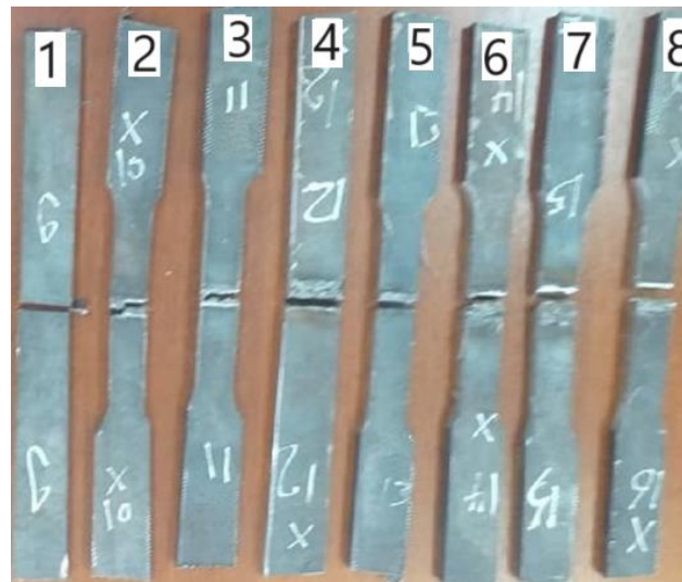
Fig.3. Weldments after tensile test showing fracture in the welds (FZ and HAZ)
