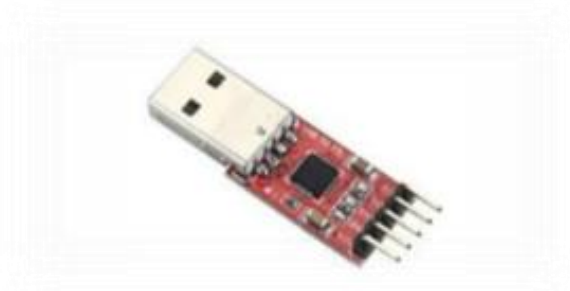
Fig. 6. USB and ttl driver.
