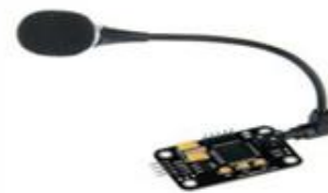
Fig. 4. Voice recognition module.
