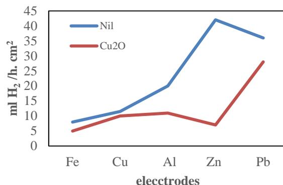
Fig.1. The effect of Cu<sub>2</sub>O for production of H<sub>2</sub> at electrodes.
