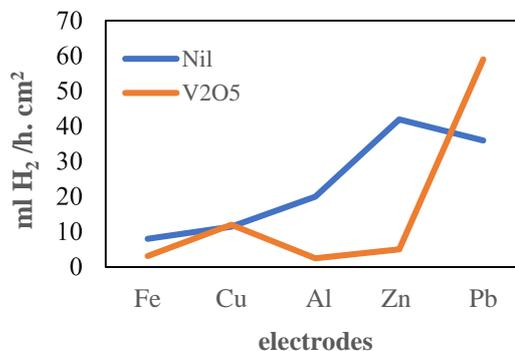
**Fig.3. The effect of V2O5 on the production of H2 at electrodes.**
