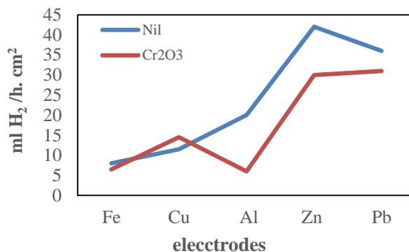
Fig.2. The effect of Cr<sub>2</sub>O<sub>3</sub> on the production of H<sub>2</sub> at electrodes.
