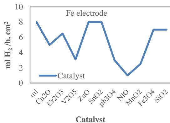
Fig.11. The effect of metal oxides at Fe electrode.
