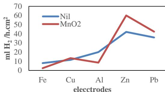
**Fig.8. The effect of MnO2 on the production of H2 at electrodes.**
