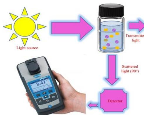
Figure 2. Turbidity measurements by 2020 Nephelometer.
