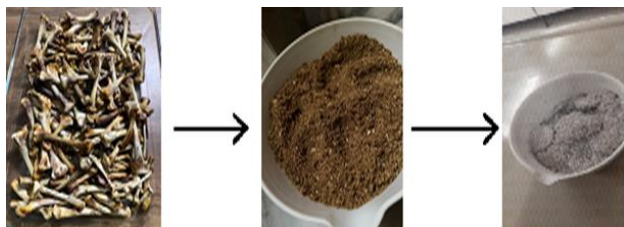
Figure 1. Stages of synthesis of the calcium oxide
