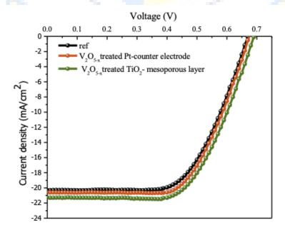
Figure 1. Current density-voltage (J-V) curves of DSSCs made with Pt counter electrode and  $TiO_2$  photoanode treated with Vanadium(V) oxide ( $V_2O_{5-x}$ )
