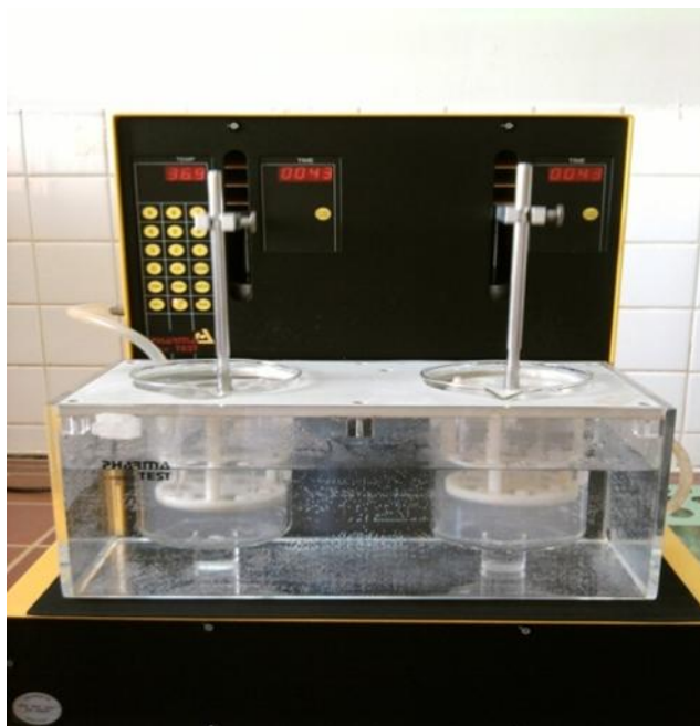
Figure 5: Disintegration test (pharma test (PTZ-E) company).
